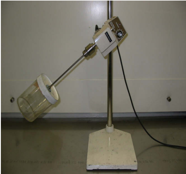
Fig. 5. Top secured overcoater used in early development stages of AGR-1 test article development.
